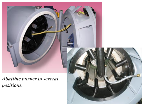
Easy disassembly of the head components.
